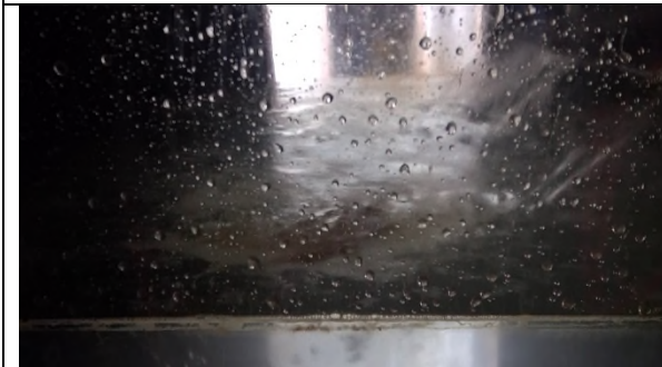
Figure C-o-247: NDB R2 S8 Oil circulation is patchy
