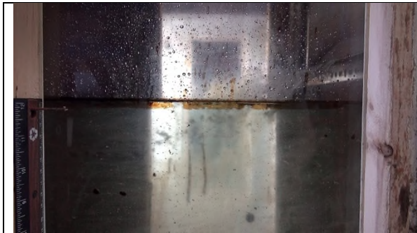
Figure C-o-66: CHV R1 S1 Non-spherical shearing, oil in column, with large neutrally buoyant droplet below.
