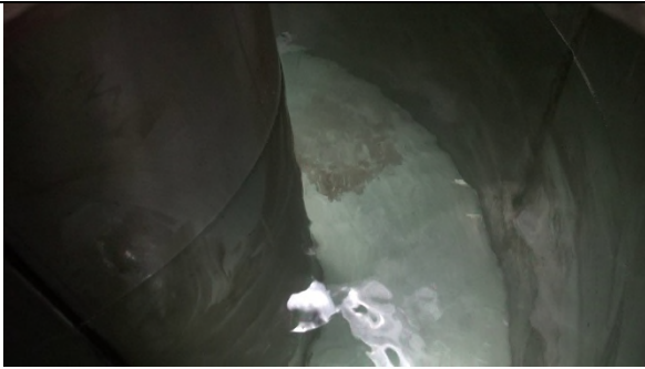
Figure C-o-9 AHS R2 S5 Oil held up near thrusters, not passing by the viewing area, no sinking detected
