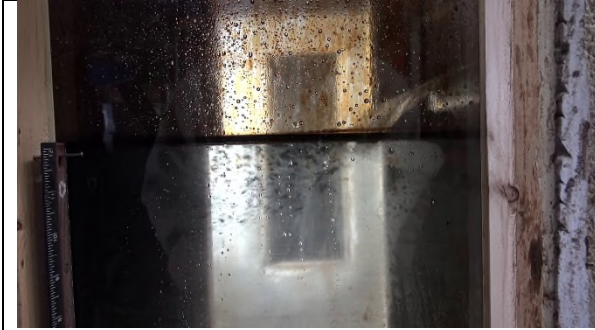
Figure C-o-170: LSB R1 S1 Small oil droplets shear off at waterfall
