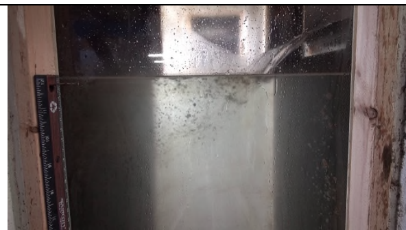
Figure C-o-278: SYN R1 S5 Oil droplets range from 1-3 mm diameter
