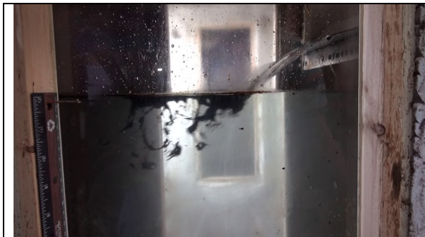
Figure C-o-1: AHS R 1 S 1 Waterfall impact on slick (streamers)
