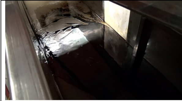
Figure C-o-180: LSB R3 S4 Oil hold-up above thruster
