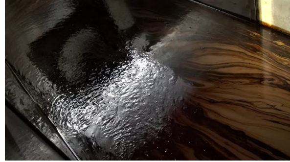
Figure C-o-265: SYB R3 S1 Oil hold-up between thruster and fan
