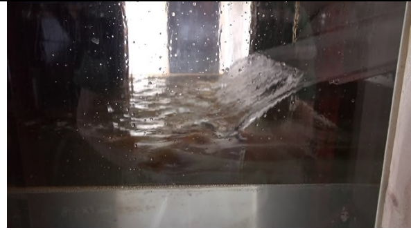
Figure C-o-284: SYN R2 S5 Oil circulating in non-contiguous patches on the water surface
