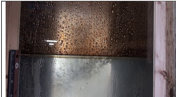
Figure C-o-176 LSB R2 S5 Oil still forms small droplets under the waterfall
