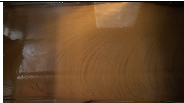
Figure C-o-246: NDB R2 S6 Emulsified oil on N side of tank
