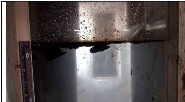
Figure C-o-3 AHS R 1 S 5 Oil collecting on sidewalls
