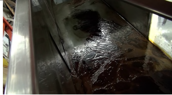
Figure C-o-171: LSB R1 S9 Oil hold-up between thruster and fan
