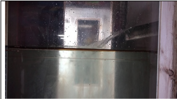
Figure C-o-289: SYN R3 S1 Column is clear, oil is very fluid
