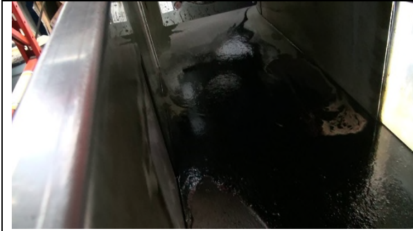
Figure C-o-49 Viscous oil resisting movement within flume
