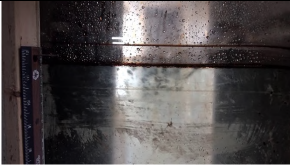
Figure C-o-252: SYB R1 S1 Spherical droplets approx 1-4 mm
