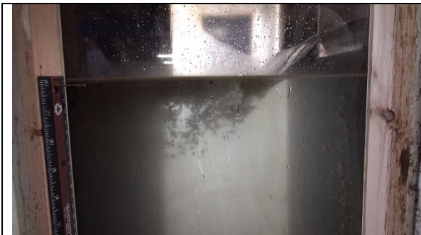
Figure C-o-279: SYN R1 S5 Large slug of oil hits waterfall results in semi-spherical droplets (oil still has low viscosity)
