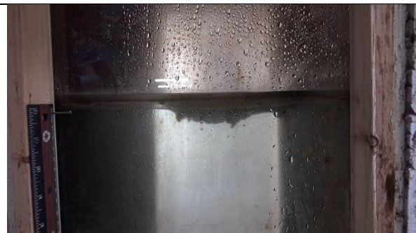
Figure C-o-173: LSB R1 S13 Oil too viscous for waterfall
