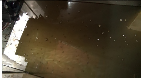
Figure C-o-121 CRW R2 S1 Some bubbles imparted from waterfall
