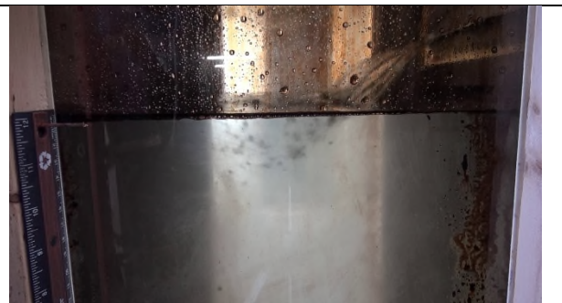
Figure C-o-200: MSB R1 S8 Waterfall still shearing oil droplets
