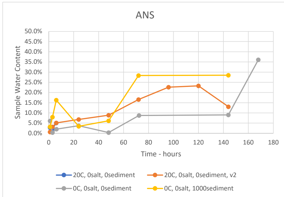
Figure C-o-4o Ultimate Water Content of ANS Flume Samples
