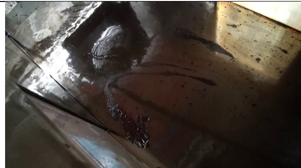
Figure C-o-44 AWB R1 S7 Usual spot for oil hold-up.
