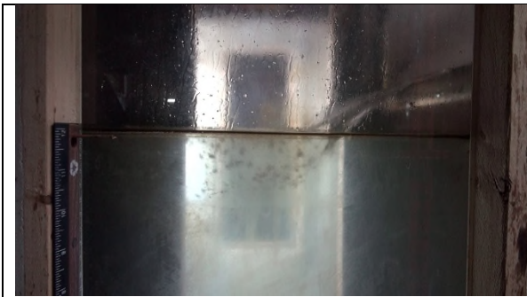
Figure C-o-116: CRW R1 S1 Oil "misting" into water column
