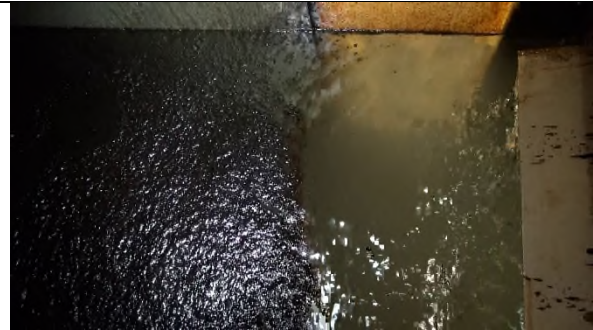
Figure C-o-237: MSW R5 S7 Oil mass moved around the tank to a spot between the waterfall and the S side fan
