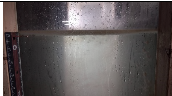
Figure C-o-280: SYN R1 S8 Oil hold-up limits circulation to thin sheen
