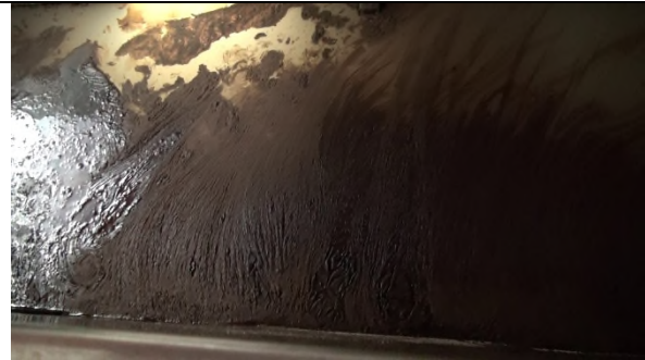
Figure C-o-267: SYB R3 S7 Oil hold-up at end of run
