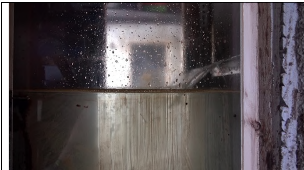
Figure C-o-245: NDB R2 S6 Some oil hold-up, reducing circulation
