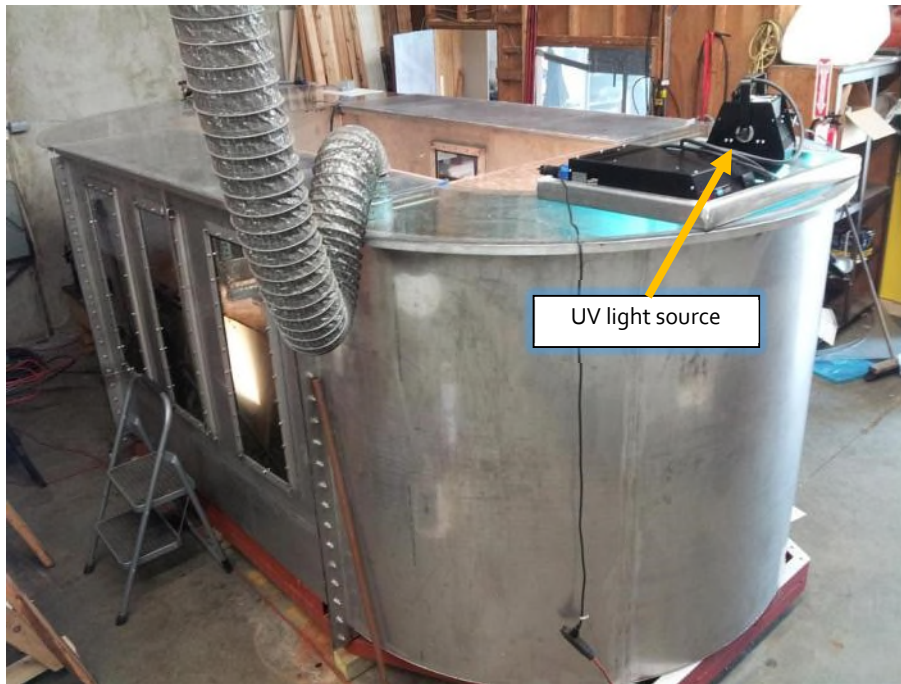
Figure 6-1: Meso-Scale Oil Weathering Tank
