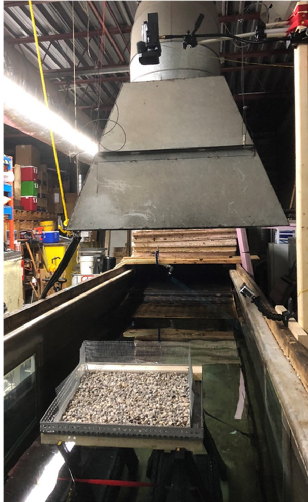
Figure 8-3: Shoreline adhesion test cell mounted in wave tank
